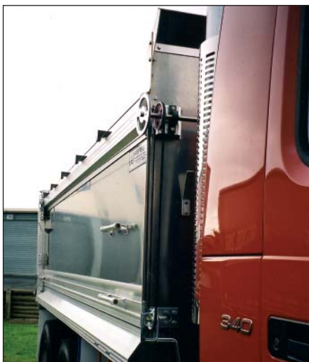
A mechanical tarping system that complies with the 2.5 metre vehicle width
