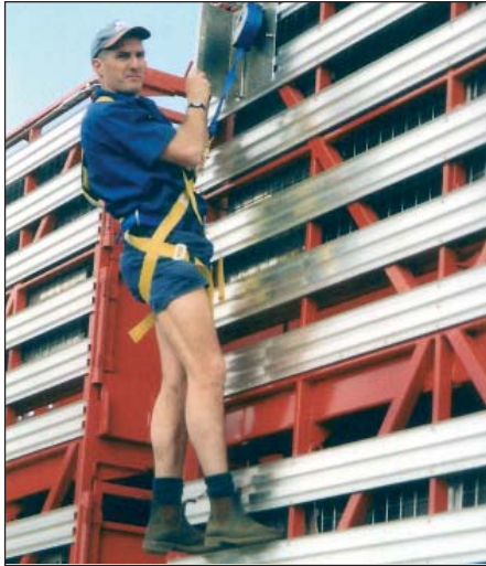
Driver using a safety harness fitted to a vehicle to attend to livestock
