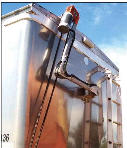
Mechanical arm to wind the tarp must be folded to the front or rear of the vehicle
